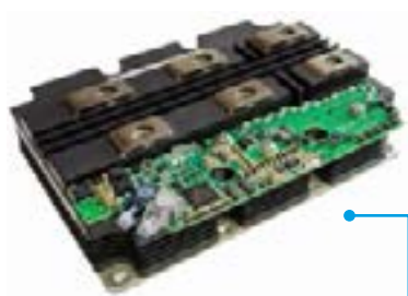
Latest generation of HV 6.5 kV IGBTs
